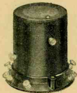
R.I. Micrion coil embodying permeability adjustment of inductance.
